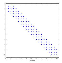
Use optimset to set the HessPattern parameter to Hstr. When a problem as large as this has obvious sparsity structure, not setting the HessPattern parameter requires a huge amount of unnecessary memory and computation. This is because fmincon attempts to use finite differencing on a full Hessian matrix of 640,000 nonzero entries.
