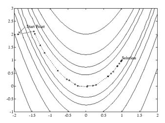
Figure 3-2: BFGS Method on Rosenbrock's Function
