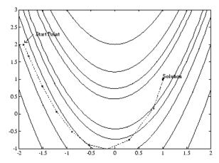
Figure 3-3: Gauss-Newton Method on Rosenbrock's Function
