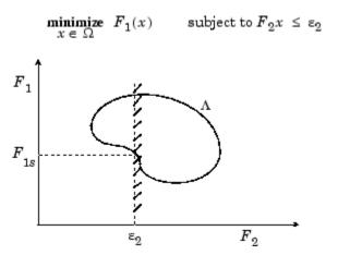
Figure 3-11: Geometrical Representation of ε-Constraint Method
